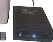
Mini bench produces hydrogen from water through an electrolyser. It can refill one cylinder in three to five hours and only requires power supply and pure water.
