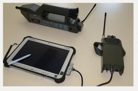
Training and Simulation Kit with control panel radio connected with AP4C
